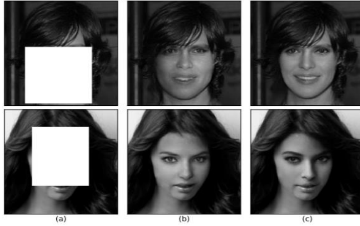
Fig. 9. (a) - the initial image for restoration, (b) - the result of the model without additional training, (c) - the result of the model with additional training with a cascade discriminator
