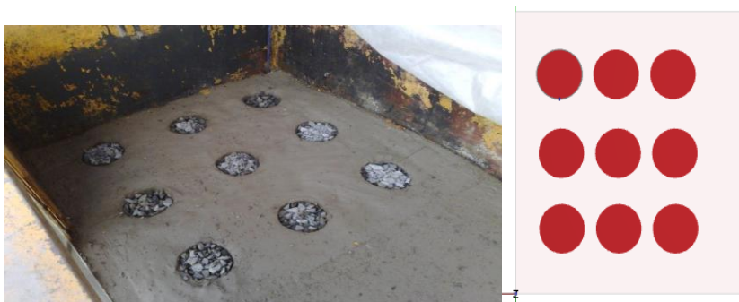
Fig. 3. Pattern of stone columns at s=2.5d
