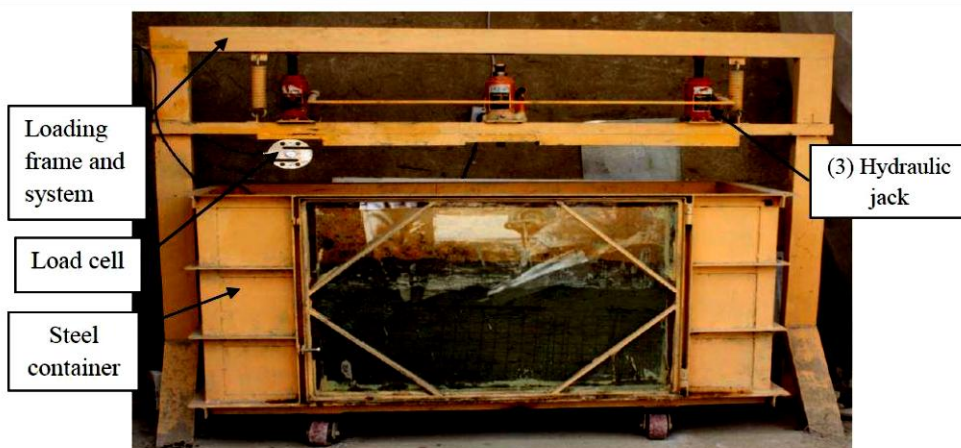
Fig. 2. Experimental test container and loading system (after Hassan, 2013)
